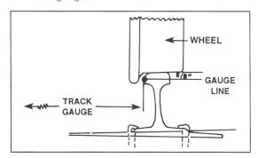
gauge line—a line <sup>5</sup>/<sub>8</sub> in. (1.59 cm) below the top of the centerline of the head of the running rail along the side that is nearer the center of the track.
