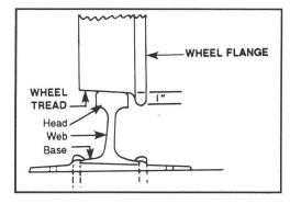
wheel tread—in rail systems, the exterior cylindrical or conical surface of a steel wheel that comes in contact with the rail.
