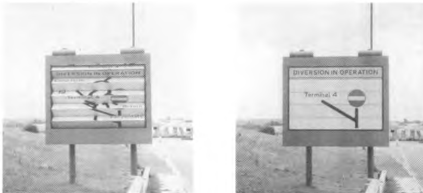
Figure 2-10. Horizontal Drum (Prism) Sign at Heathrow Airport in London
