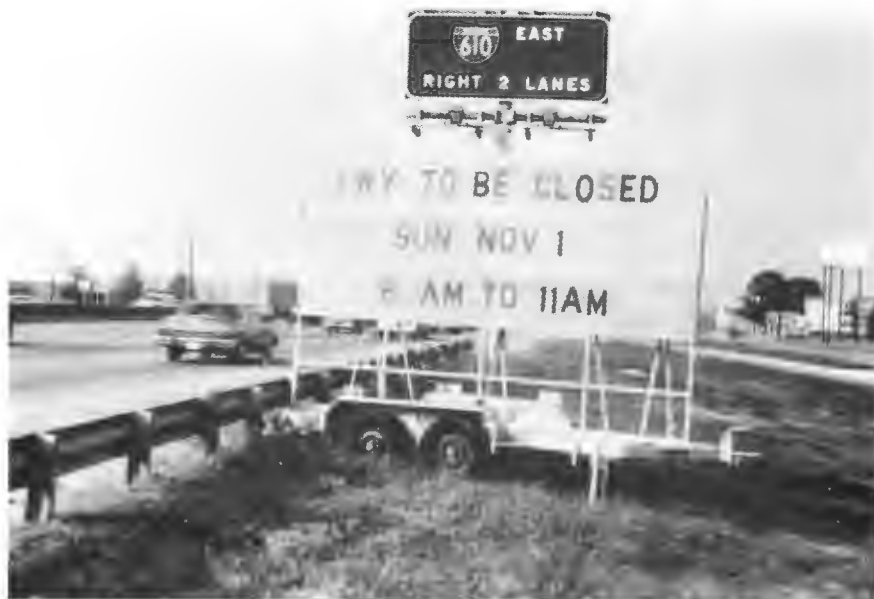
Figure 2-52. Trailer-Mounted Changeable Message Sign, Texas State Department of Highways and Public Transportation
