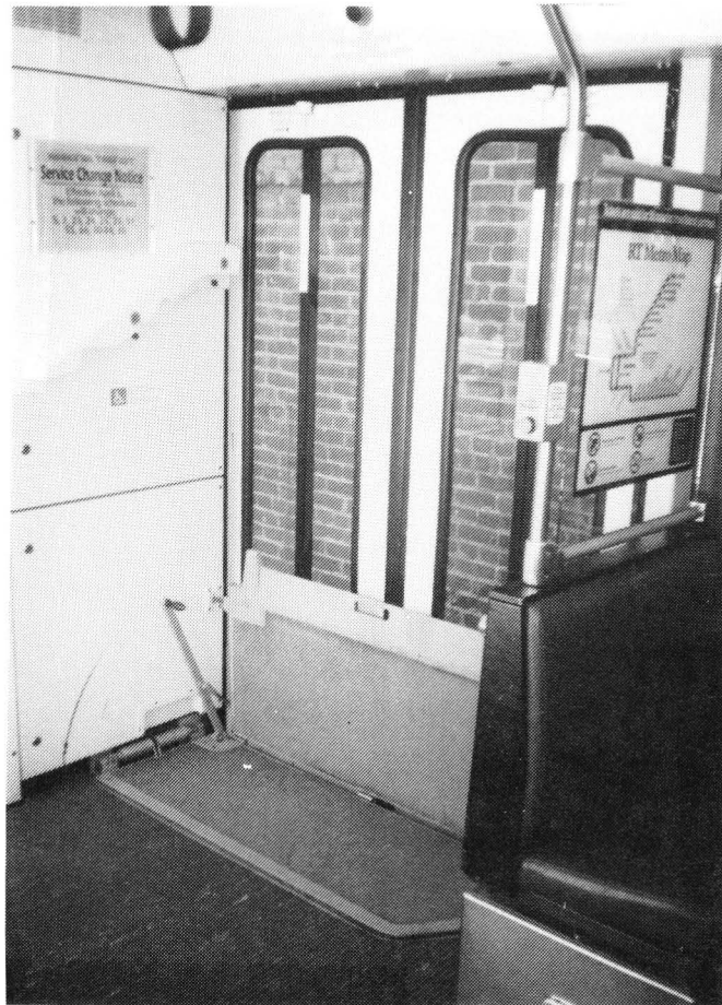
FIGURE 2-17. PARTIALLY DEPLOYED POSITION OF SACRAMENTO BRIDGING DEVICE USED DURING NORMAL OPERATION
