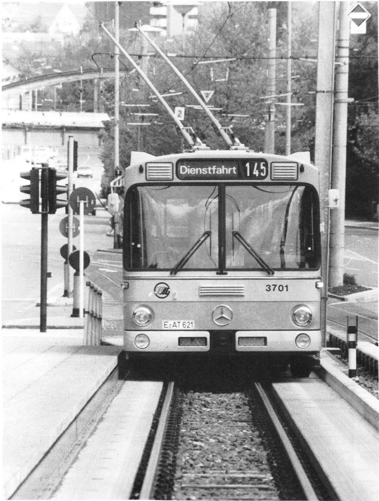
FIGURE 5-8. GUIDED BUS IN ESSEN, GERMANY
