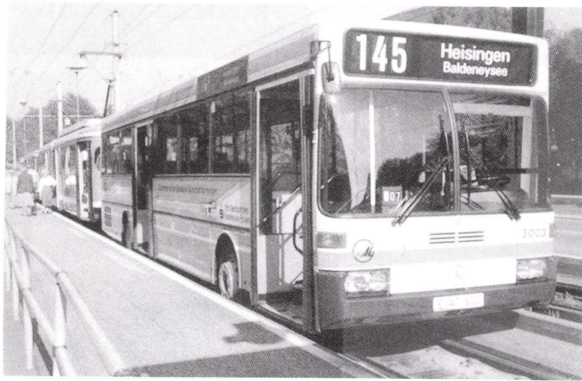
FIGURE 5-12. ESSEN PLATFORM IS LEVEL WITH FIRST STEP OF GUIDED BUS
