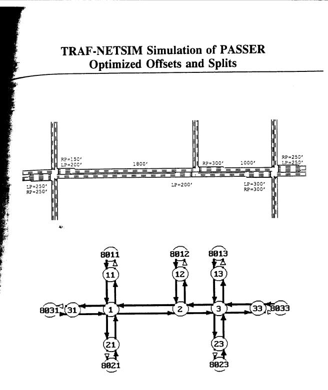
This is the same arterial network as used in the PASSER and TRANSYT sample problem and is the simulation of PASSER's optimized offsets and splits.
