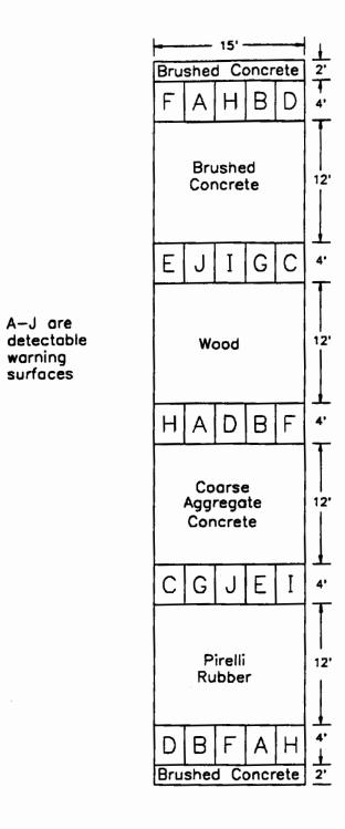
Figure 2-1. Laboratory platform for testing detectability of ten detectable warning surfaces in association with four platform surfaces; Phase I (modified for Phase II). Located at old Broadway Station, MBTA.
