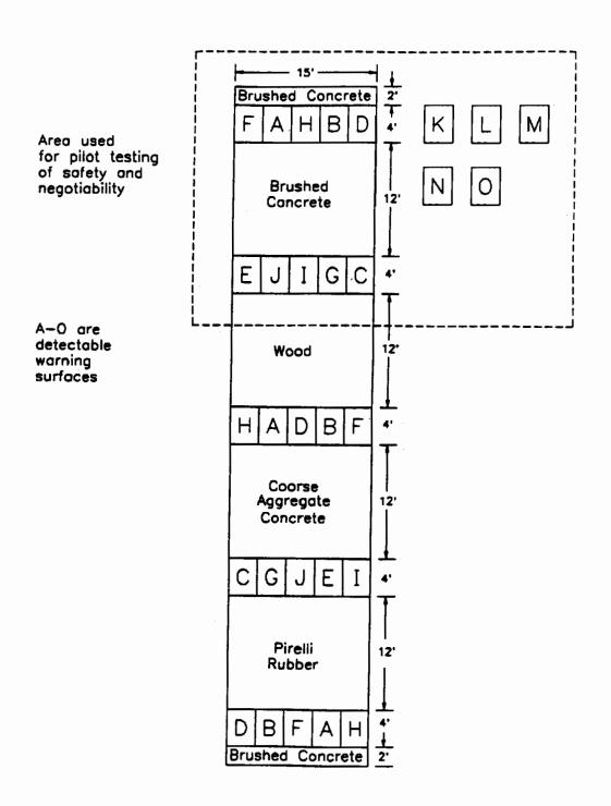
Figure 4-1. Laboratory platform for testing detectability of ten detectable warning surfaces when approached from four platform surfaces. Figure shows portion of platform and adjoining level floor used for pilot testing of safety and negotiability. Constructed at old Broadway Station, MBTA.
