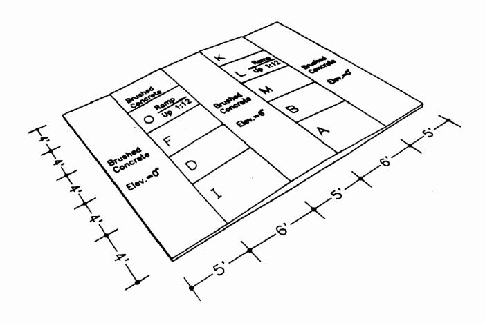
Figure 5-1. Laboratory ramps for testing safety and negotiability of nine detectable warnings on slopes (1:12). Constructed at old Broadway Station, MBTA.
