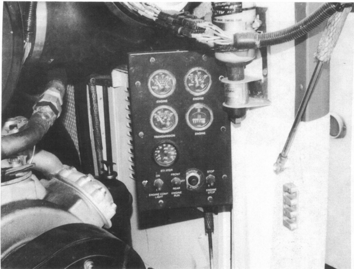
PHOTOGRAPH 2-13 IKARUS USA ARTICULATED MODEL: ENGINE COMPARTMENT CONTROL BOX CONTAINING ENGINE STOP SWITCH
