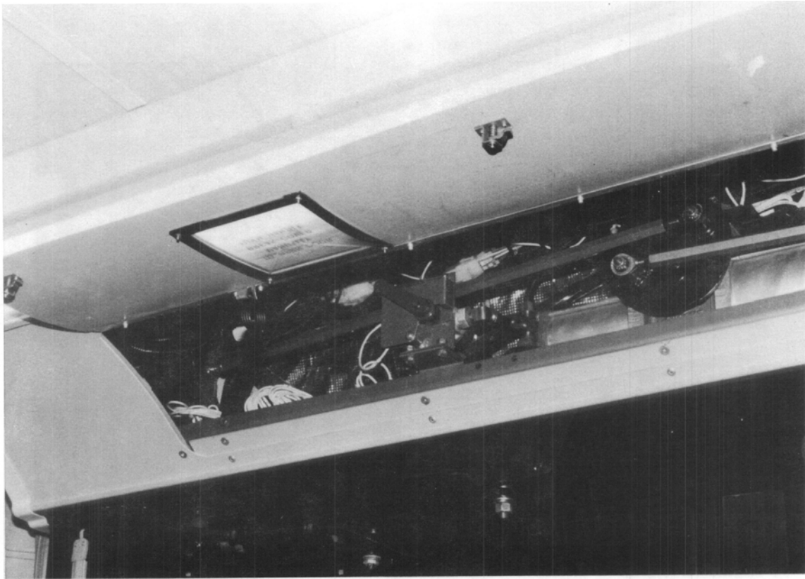
PHOTOGRAPH 2-47 IKARUS USA ARTICULATED MODEL: LOCATION OF REAR DOOR DUMP VALVE OVER REAR DOORS
