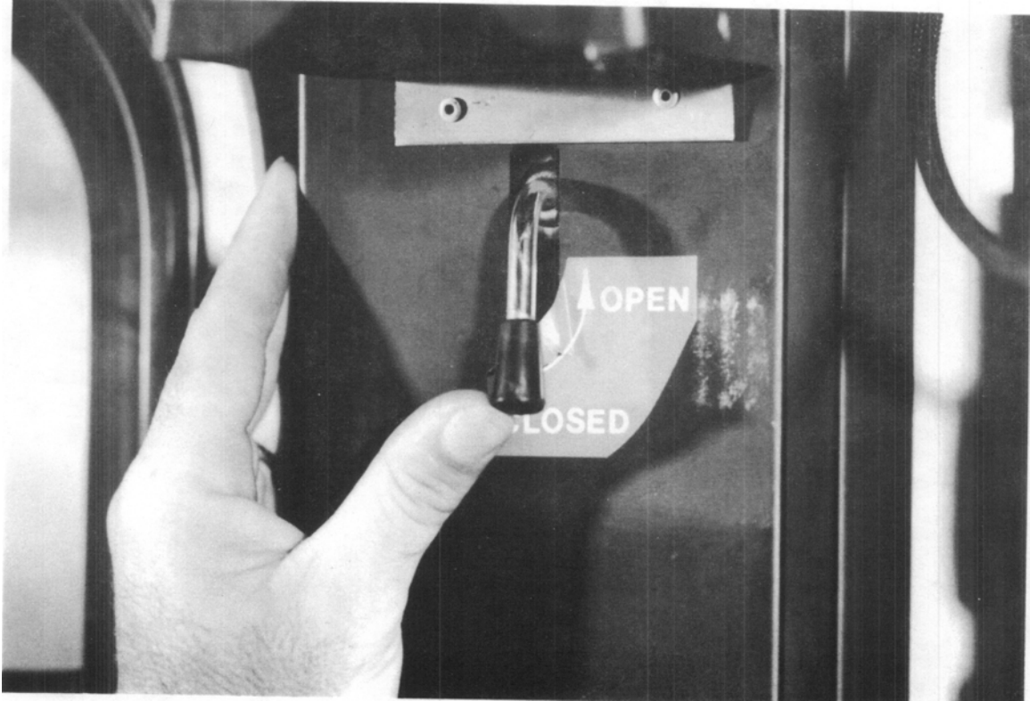
PHOTOGRAPH 2-49 NEOPLAN USA MODEL: EMERGENCY REAR DOOR DUMP VALVE
