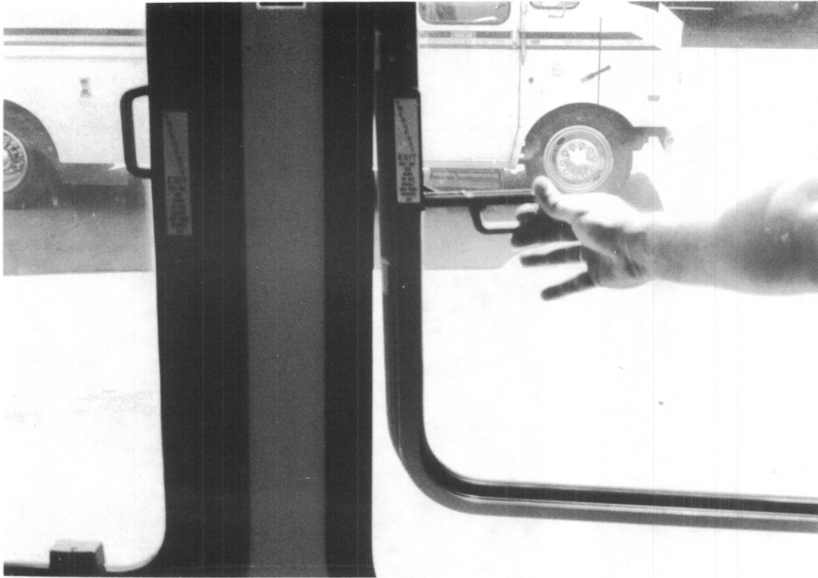
PHOTOGRAPH 2-61 GILLIG PHANTOM MODEL: USE OF EMERGENCY RELEASE FOR EMERGENCY PASSENGER SIDE WINDOW
