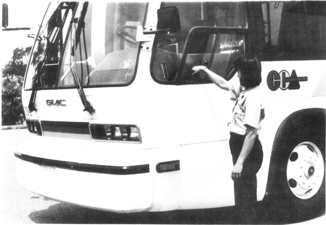
PHOTOGRAPH 2-34 GMC RTS MODEL: USE OF DOOR DUMP VALVE AT OPERATOR'S SIGNAL WINDOW
