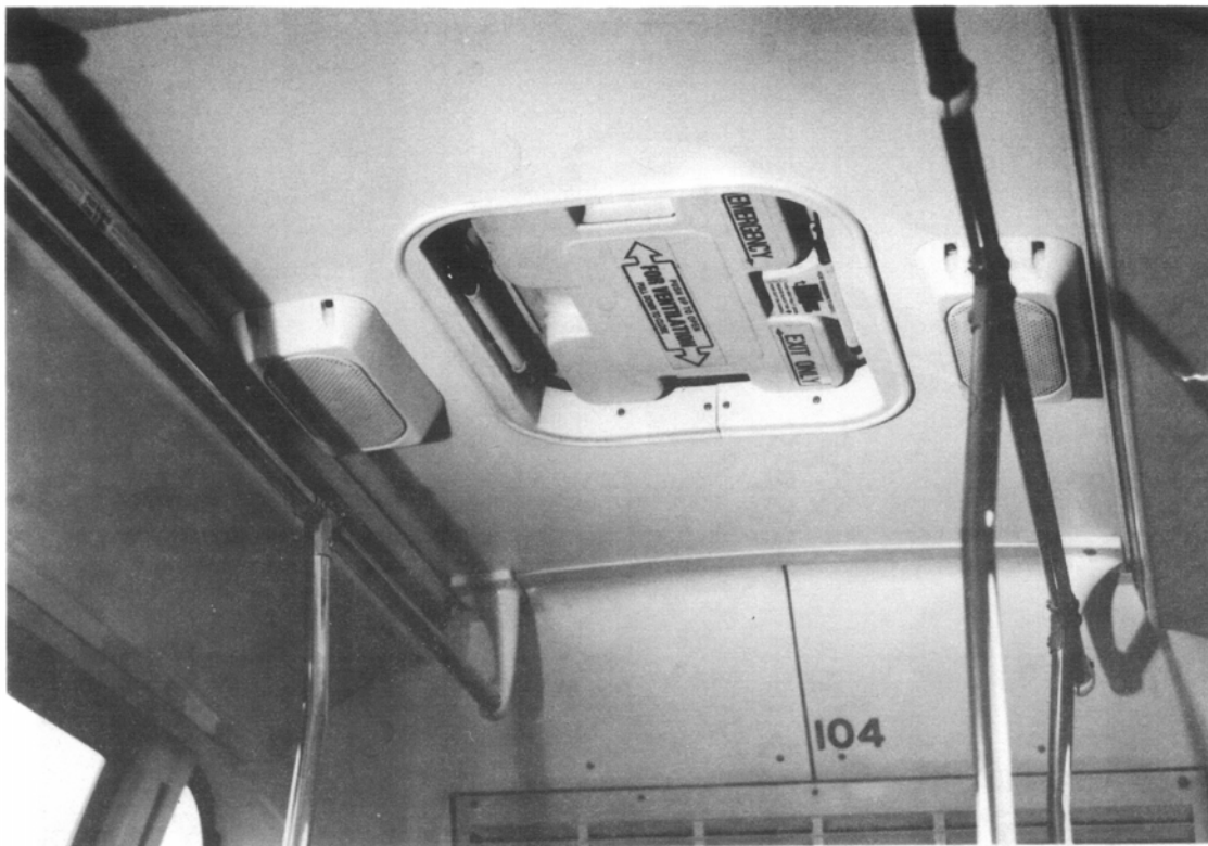
PHOTOGRAPH 2-24 GMC RTS MODEL: INTERIOR VIEW OF ROOF ESCAPE (INGRESS) HATCH WITH STREET SIDE ORIENTATION
