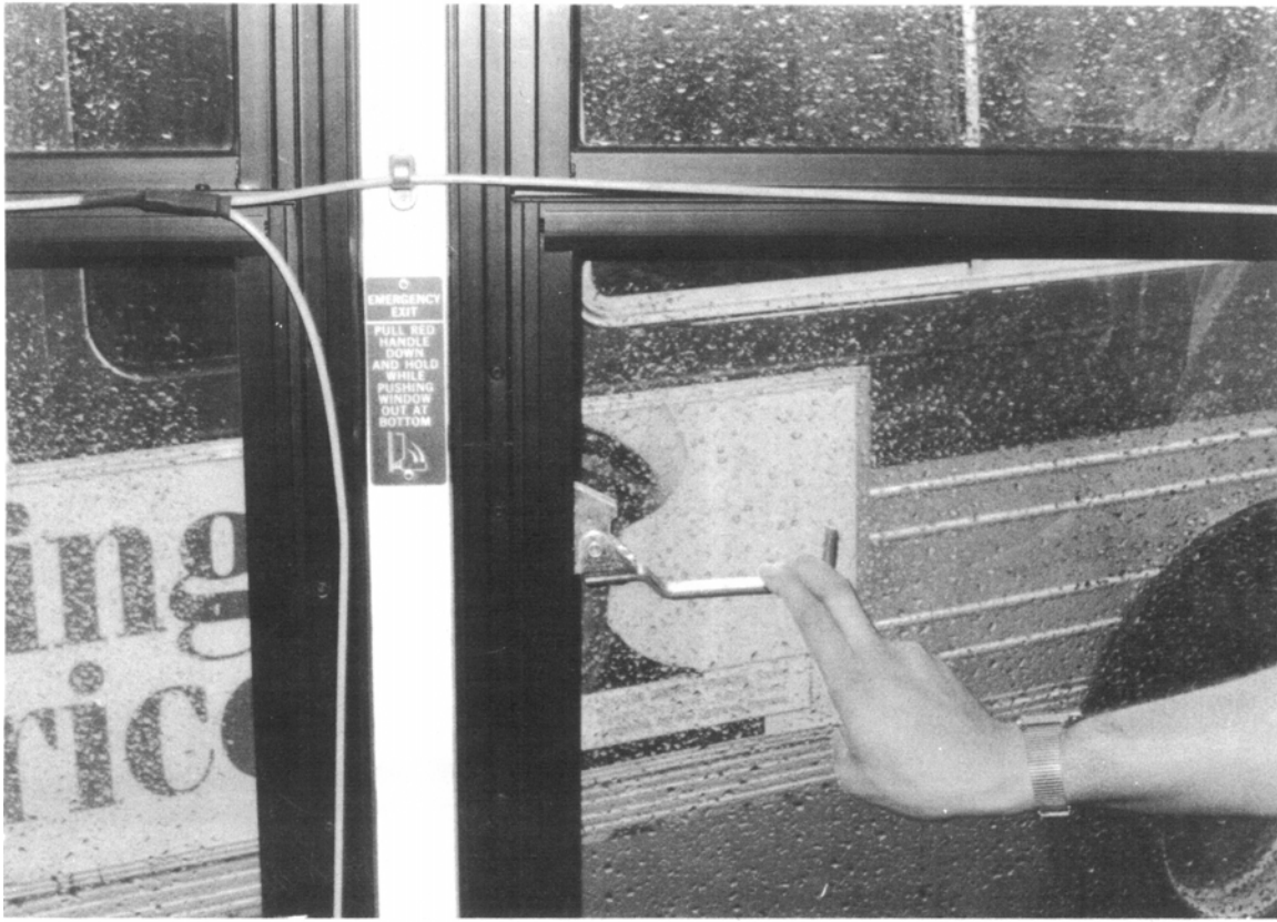
PHOTOGRAPH 2-62 IKARUS USA ARTICULATED MODEL: USE OF EMERGENCY RELEASE FOR EMERGENCY PASSENGER SIDE WINDOW
