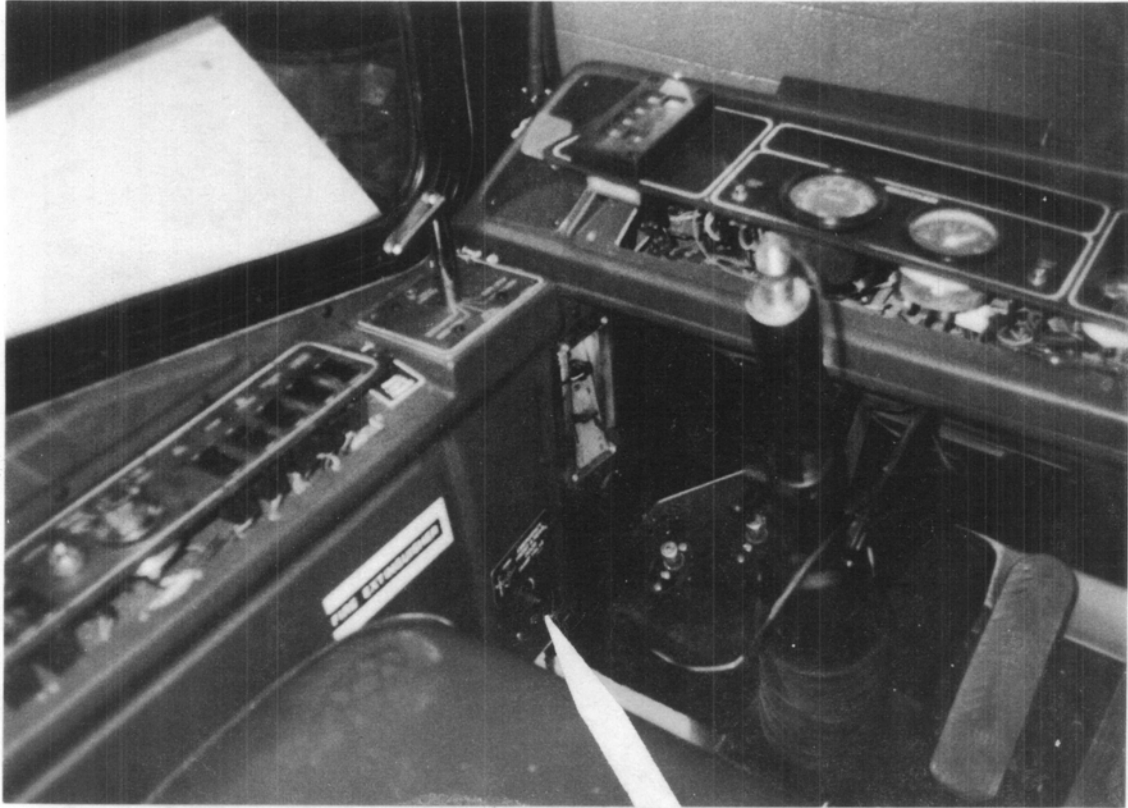
PHOTOGRAPH 2-37 NEOPLAN USA MODEL: LOCATION OF DRIVER'S AREA DOOR DUMP VALVE BELOW DOOR CONTROL HANDLE
