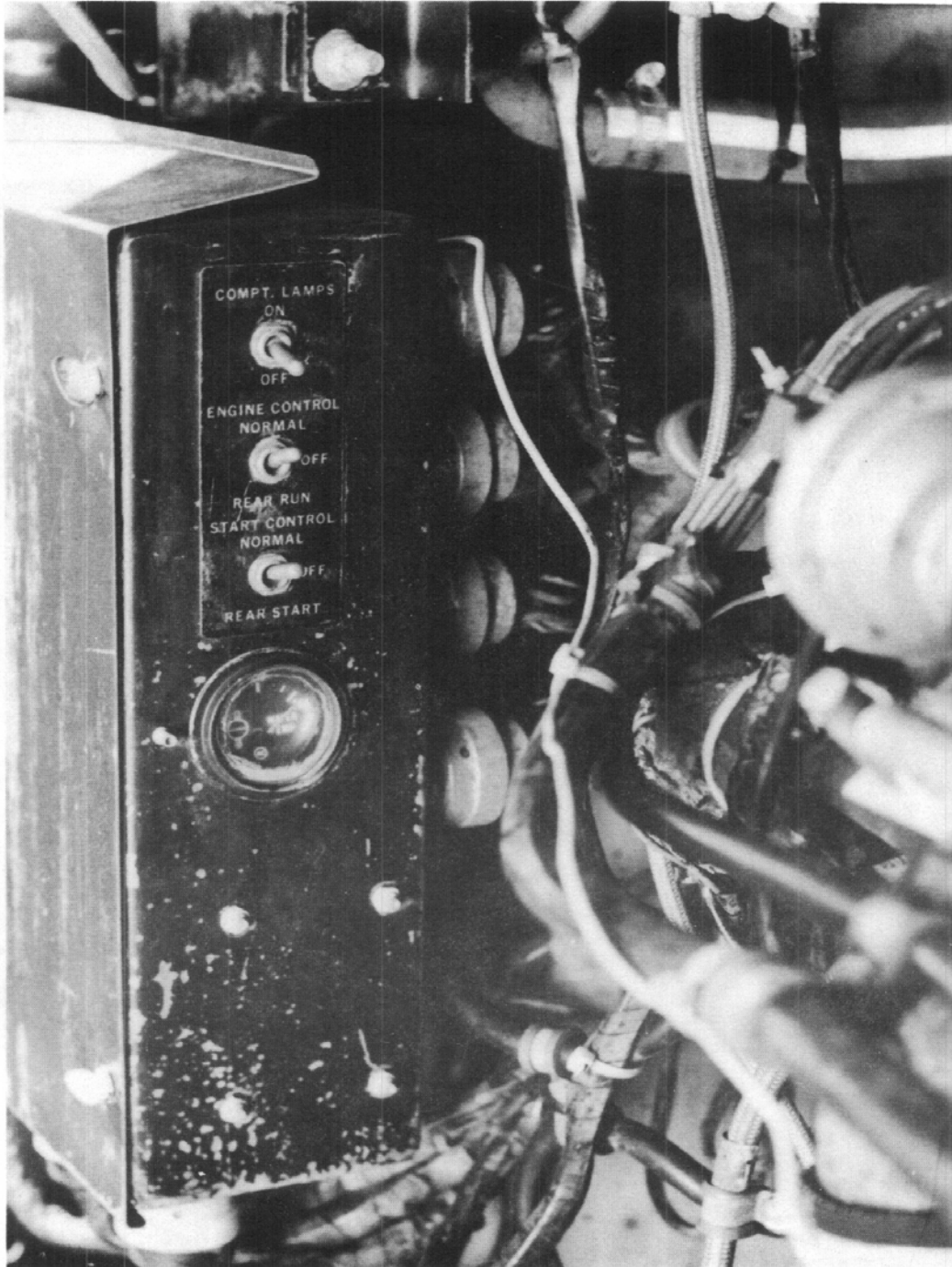
PHOTOGRAPH 2-10 FLXIBLE MODEL: ENGINE COMPARTMENT CONTROL BOX CONTAINING ENGINE STOP SWITCH
