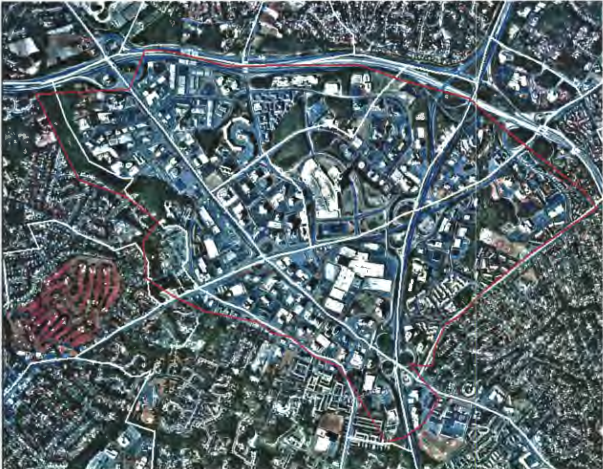
Figure 9-2 Transportation analysis zones (TAZs) in white overlaid on 1 meter DOQ imagery surrounding the Tyson's Corner, VA activity center (in red).
