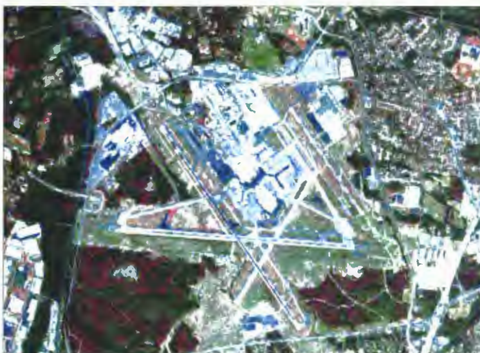
Merge product of Baltimore-Washington Airport Figure 4-3. Resolution merge enhances the spatial resolution of low resolution multispectral imagery
