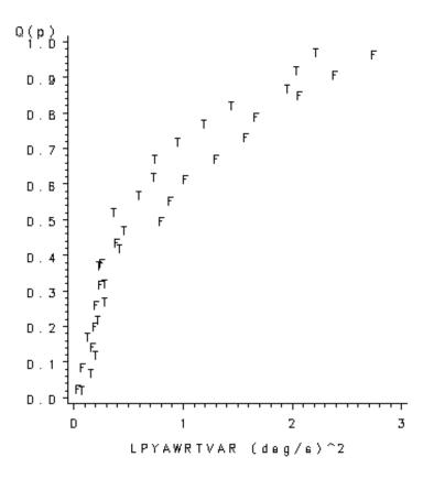
Figure 3. Empirical Quantile Plot of Low-Pass Filtered Yaw Rate Variance (LPYAWRTVAR), by False Positive (F) epochs and True Negative (T) epochs, for Test Participant 3
