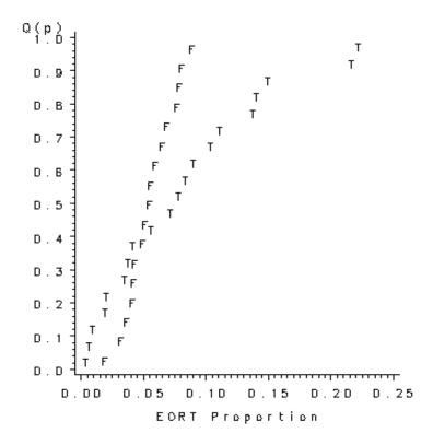
Figure 4. Empirical Quantile plot of Eyes-Off-Road-Time proportion, by False Positive (F) epochs and True Negative (T) epochs, for Test Participant 3
