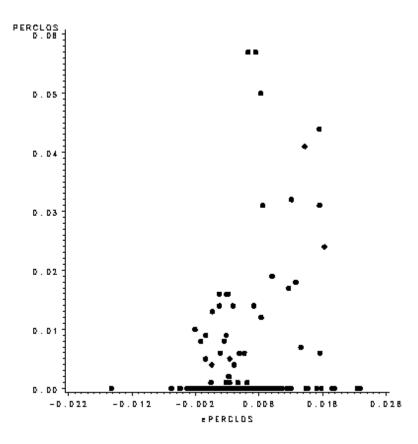
Figure 1. Scatter Plot of observed PERCLOS versus estimated PERCLOS (ePERCLOS) calculated from algorithm F4e-3, N =283 3-minute epochs from 7 test participants.
