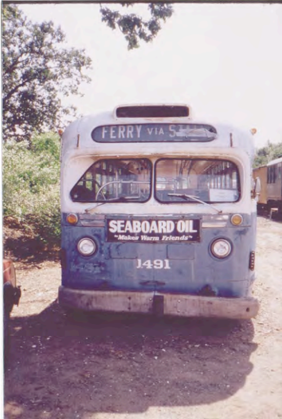
The tilted window reduced inside glare for the driver. The metal on the left was to accommodate the door. (Photo J) [23]
