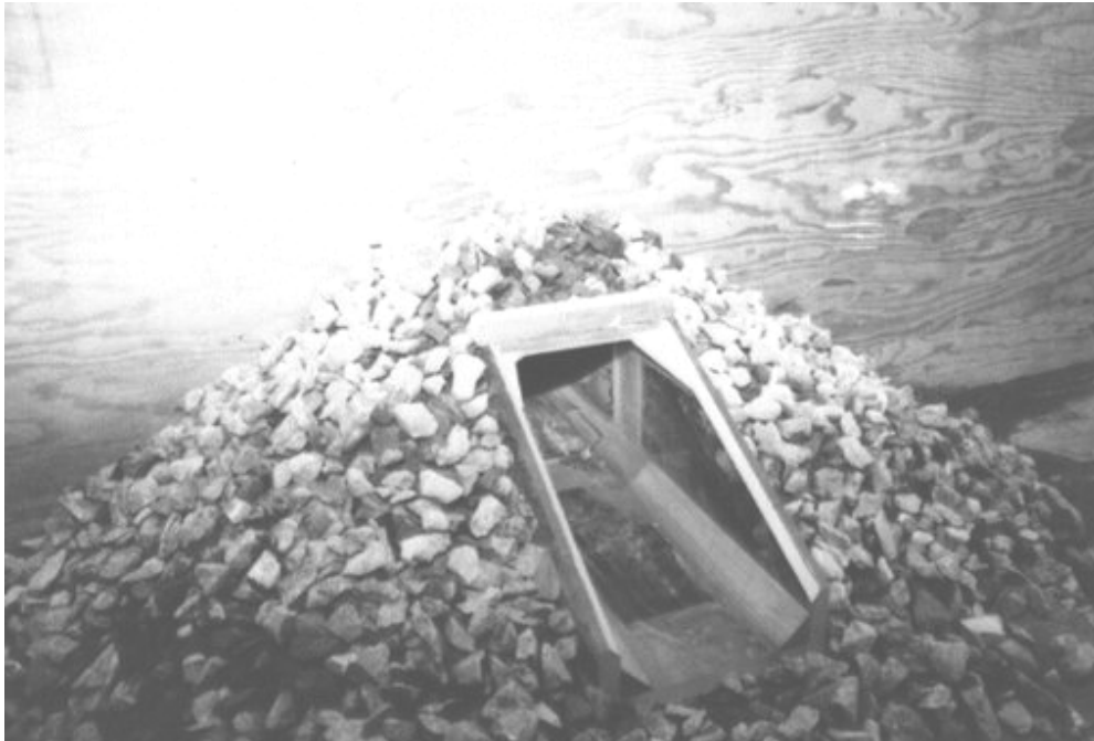
Figure 9. Culvert model 5, 6 ft x 6 ft precast, 0-degree wingwall flare.
