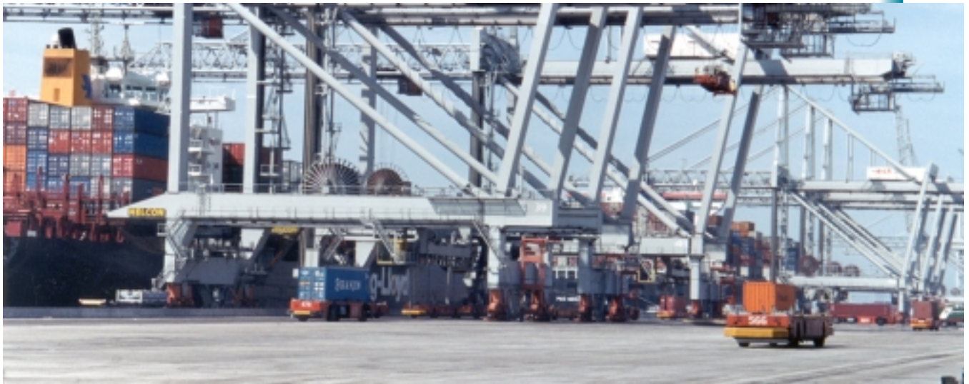
ECT container port in Rotterdam: Robot haulers unload container ship.
