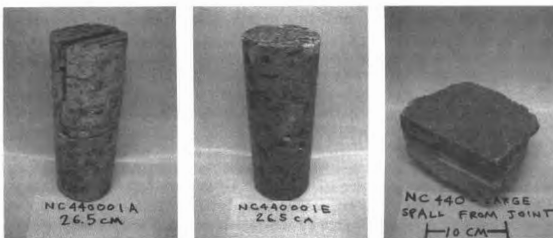
Figure 3-47. Cores and specimens evaluated from NC-440-015.
