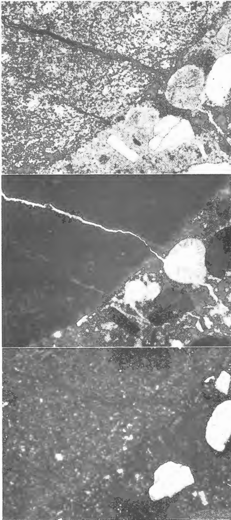
Figure 3-13. Core SD-090-019-001B, thin-section micrographs of same volcanic aggregate that was stained with sodium cobaltinitrite ASR stain as shown in figure 3-8 (c). From top to bottom: transmitted plane polarized light, epifluorescent mode, and transmitted cross polarized light. Ettringite can be seen filling the entrained air void, ASR gel can be seen in the crack within the aggregate, and hydrocalumite can be seen in the small entrained air void in the lower right hand corner. This same area was analyzed with the SEM to collect quantitative chemical information about the gel, ettringite, and hydrocalumite.
