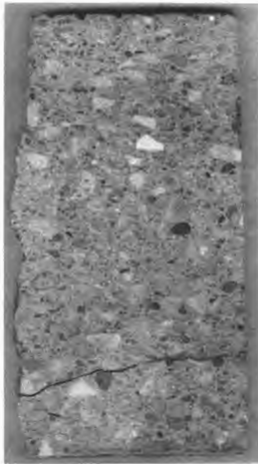
Figure 3-83. Polished slab from core IA-002-002-001A. The irregular surface along the left-hand side of the core is a cross-sectional view of the transverse joint texture.
