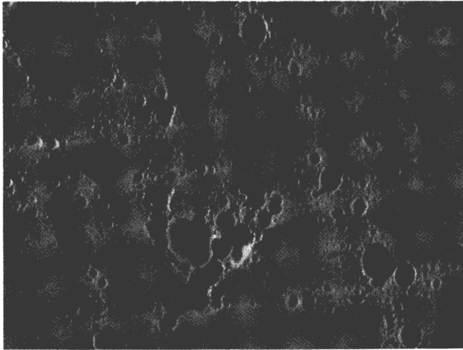
Figure 3-84. Stereo micrograph showing air void structure of IA-002-002-001A, magnified 7.5x.
