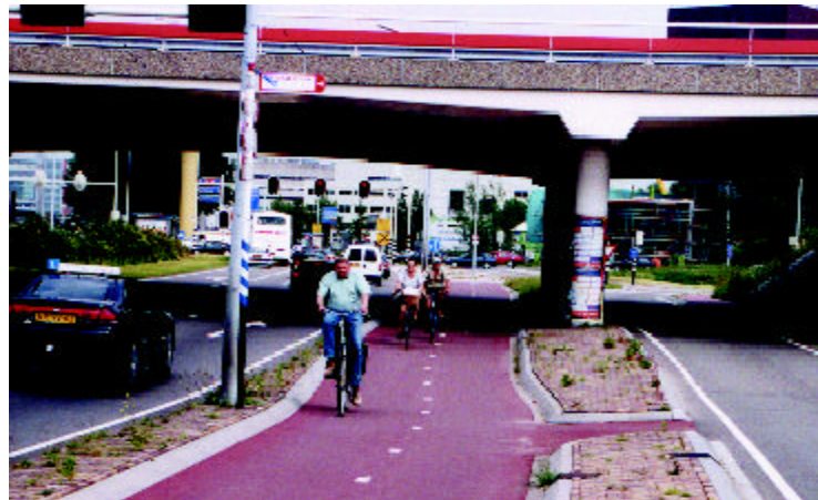
Traffic calming and context-sensitive design techniques in Phoenix, such as lane narrowing and bicycle lanes, use the roadway itself to reduce traffic speeds instead of police enforcement.
