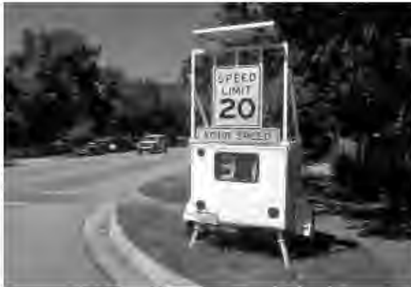
Speed-monitoring trailers let motorists know the speed limit and the speed they are traveling.
