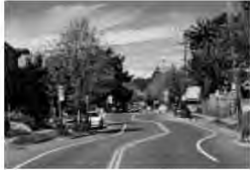
A chicane slows the speed of cars.
