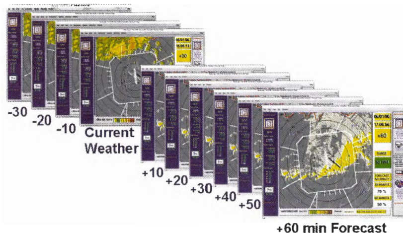
Figure 6. Succession of screenshots from the Terminal Convective Weather Forecast (TCWF), showing forecast convective weather for a local area.
