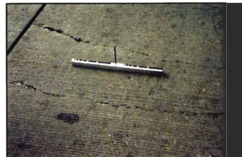
FIGURE 124 Distress Type CRCP 12—Low Severity Punchout
