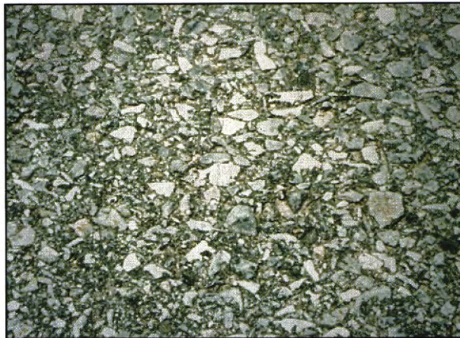
FIGURE 39 Distress Type ACP 12—Polished Aggregate
