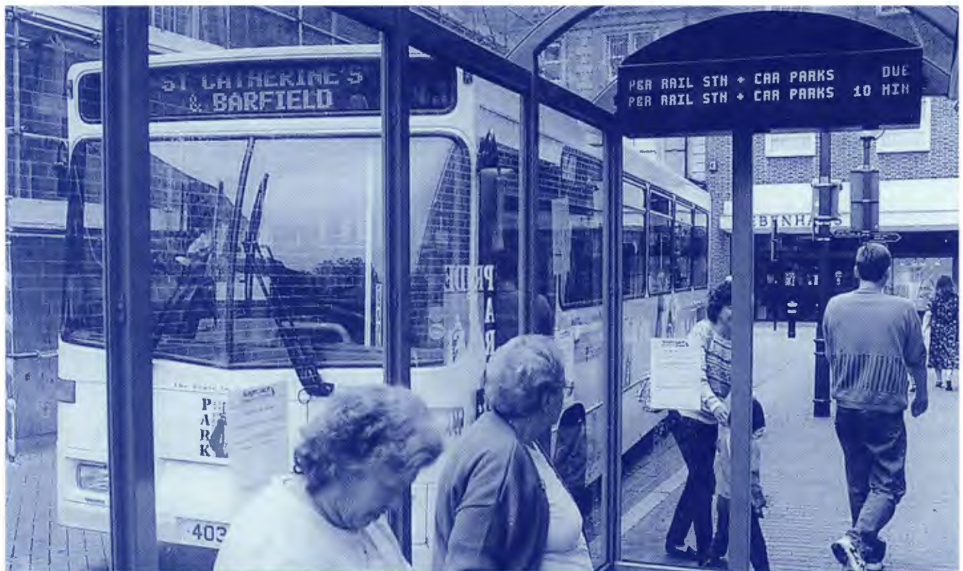
Figure 7. STOPWATCH signs provide real-time information at bus stops in Southampton and Winchester, United Kingdom. (Courtesy ROMANSE II Executive Summary)
