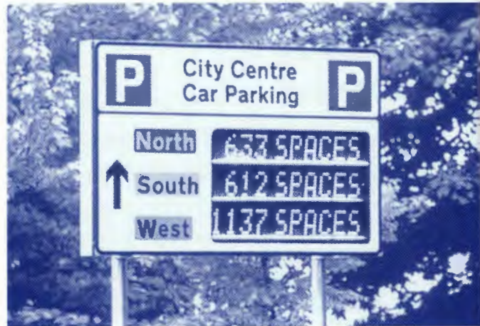
Figure 10. Variable message signs in parking lots tell drivers where empty spaces are located. (Courtesy ROMANSE II Executive Summary)
