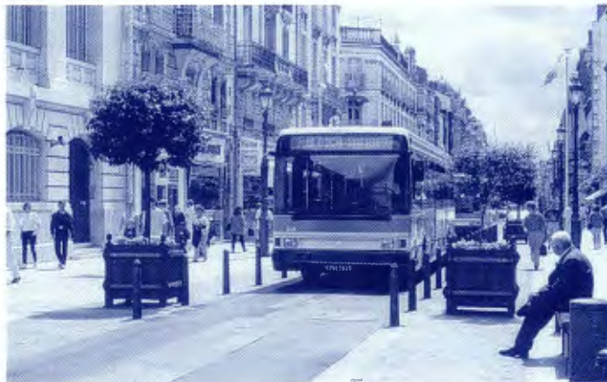
Figure 16. A dedicated bus right-of-way for buses in Orléans, France, contributes to smoother bus flows. (Courtesy Urban Transport Equipment )
