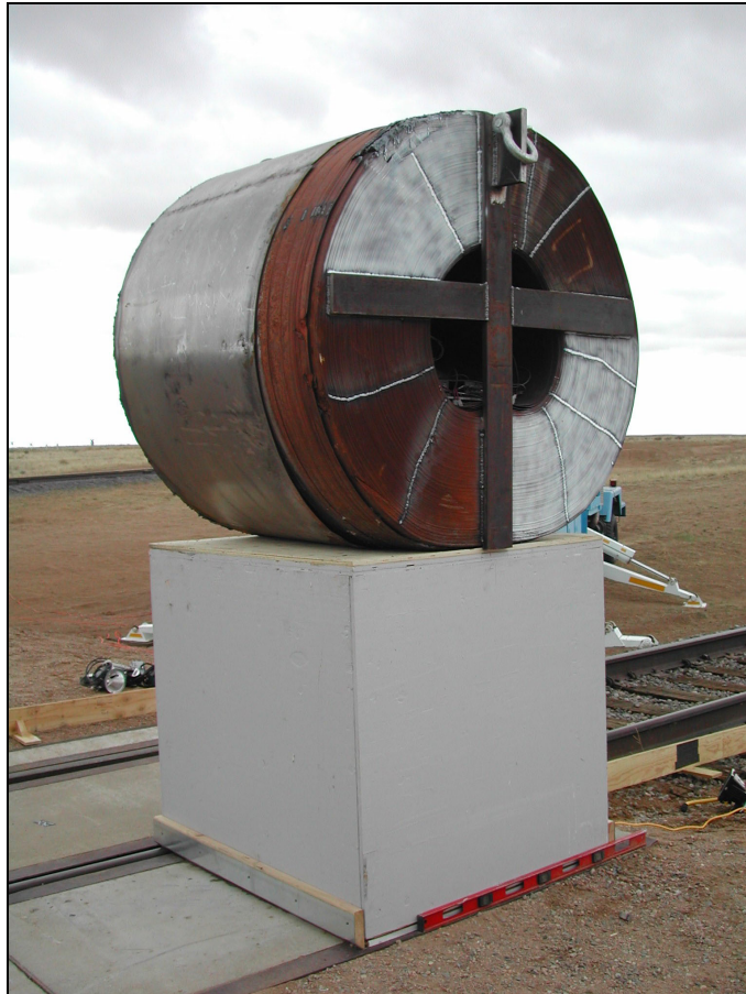
Figure 3. Steel Coil on Frangible Support
