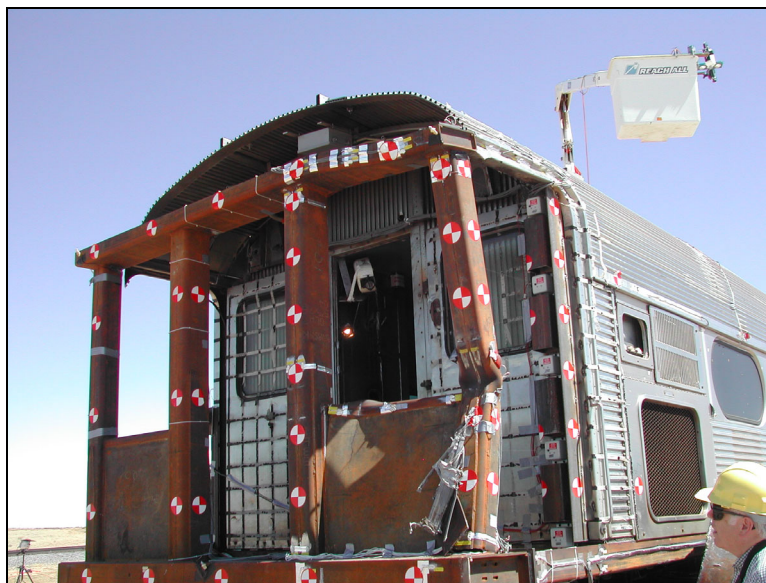
Figure 10. SOA Design Cab Car After Impact With Steel Coil
