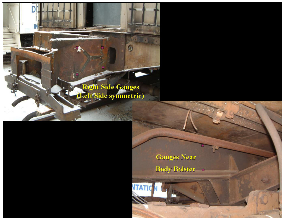
Figure 3. Placement of Strain Gauges on Draft Sill
