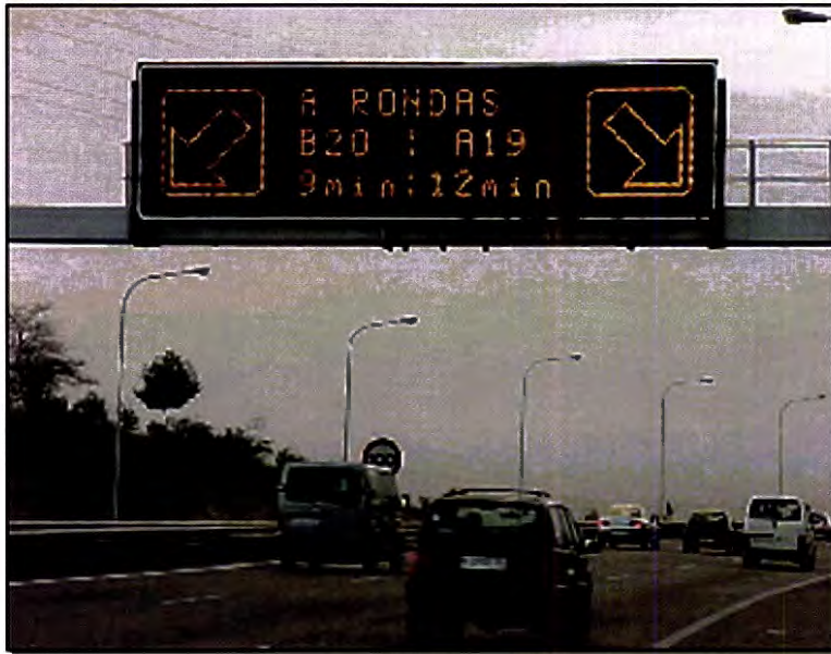
Figure 9. Dynamic message sign showing alternate travel times.
