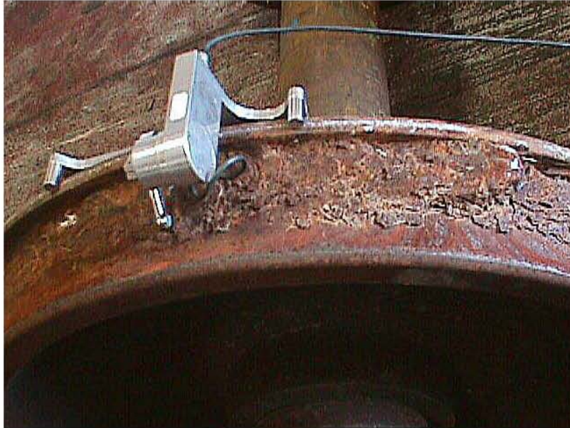
Figure 1. Built-up Metal on the Tread of a Wheel
