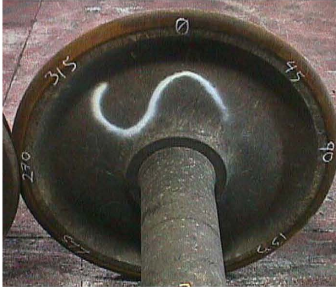
Wheel #50469 a tread damaged wheel at Progress Wheel Shop
