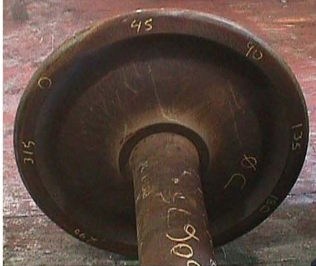
Wheel #10989 a tread damaged wheel at Progress Wheel Shop
