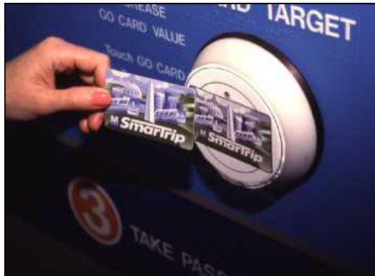
Fare Collection – Smart Card on a ticket vending machine (TVM) target
