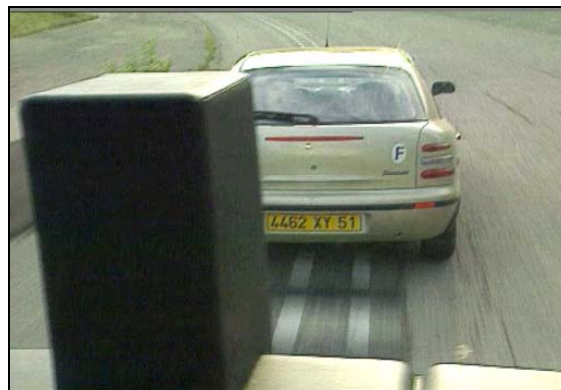
Running Way – Guidance Optical Guidance Markers in Rouen France, View through Windshield of a Vehicle following a car
