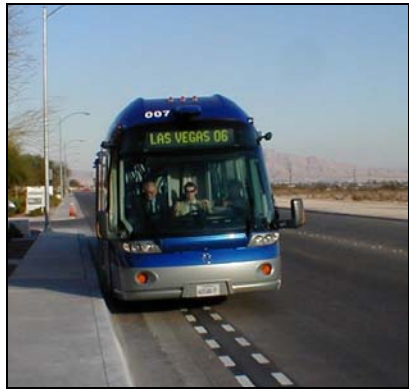
Running Way – Guidance Vehicle following Optical Guidance Markers on a test track in Las Vegas
