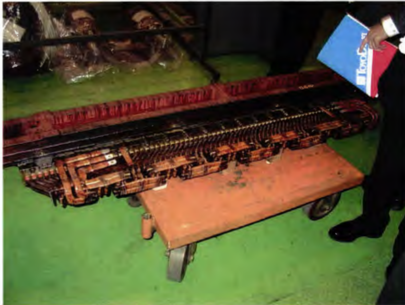
Figure A.1.9: Linear induction motor coils after being removed from the oven used for varnish curing at the Toyo Denki manufacturing plant in Yokohama.
