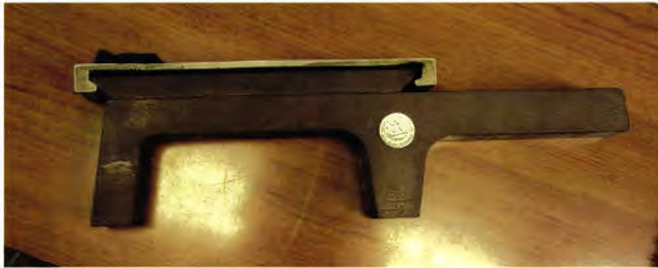
Figure 100: Cross section of the HSST structural steel and aluminum reaction rails. A U.S. quarter is laying on top of the rail for scale purposes.
