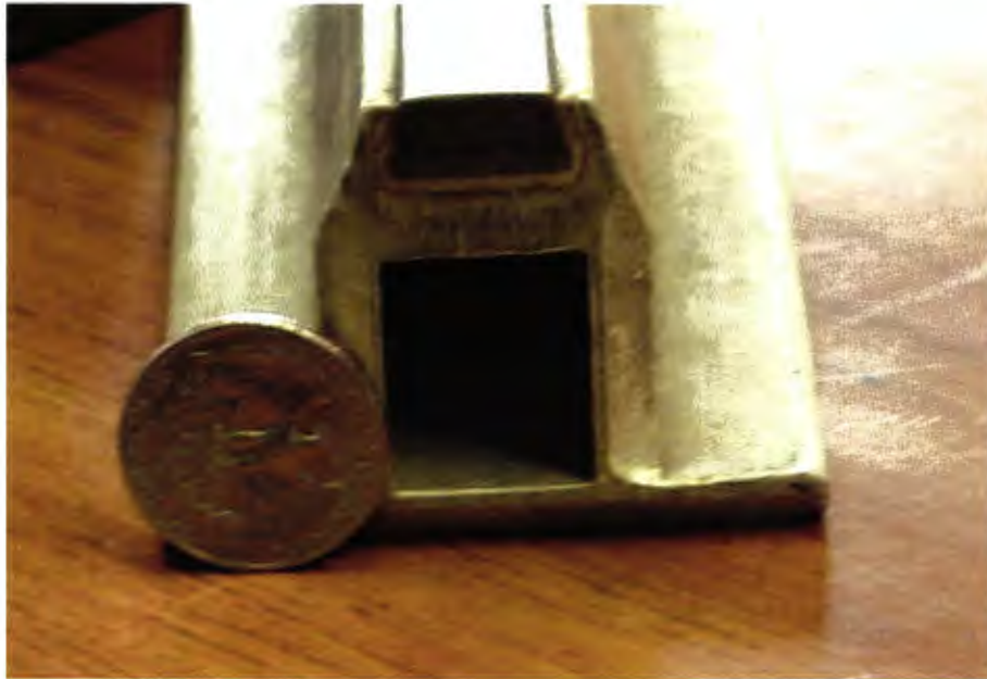
Figure 101: Cross section of the HSST electrified third rail. A U.S. quarter dollar coin is positioned next to the rail for scale purposes.
