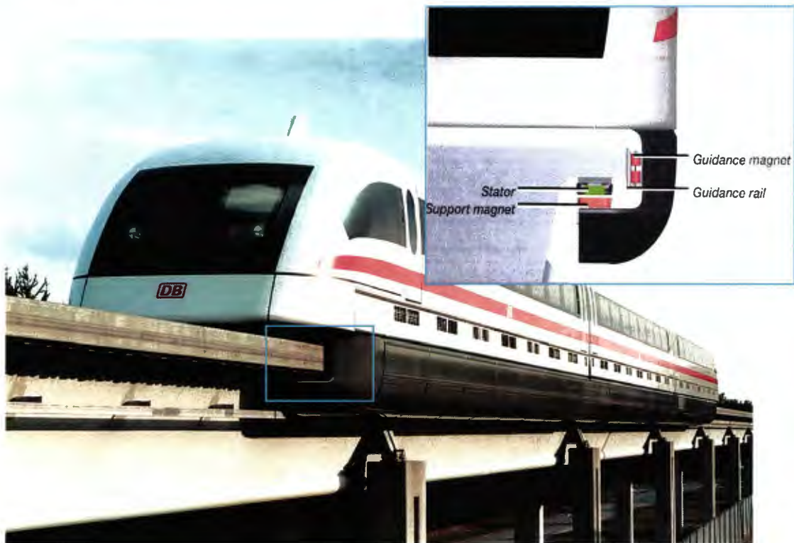
Figure 89: Transrapid TR08 vehicle and close-up of propulsion/levitation module containing on-board exciting magnets for LSM
