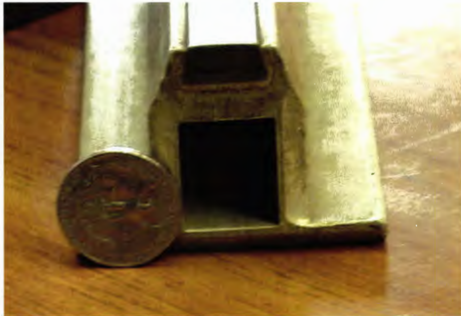
Figure A.1.4: Cross section of the HSST electrified third rail. A U.S. quarter dollar coin is positioned next to the rail for scale purposes.
