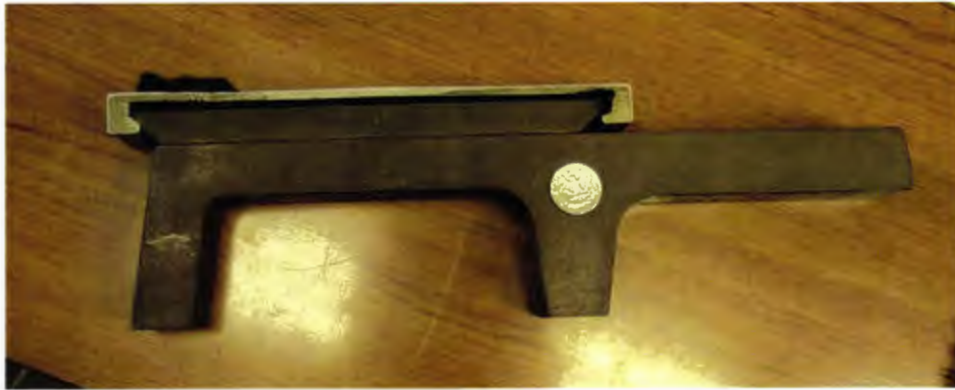
Figure A.1.3: Cross section of the HSST structural steel and aluminum reaction rails. A U.S. quarter dollar coin is positioned on top of the rail for scale purposes.
