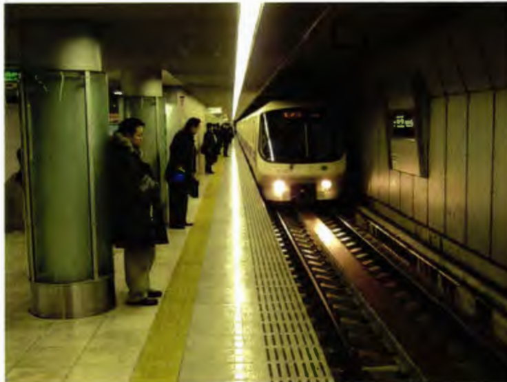
Figure A.1.7: Tokyo's newest subway, the OEDO line has a linear induction propulsion system. The copper reaction rail (located between the two guidance rails) is explosively welded to a steel substrate.
