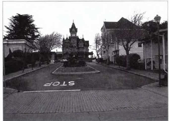
Looking down Second Street from L Street showing bulb-outs, brick crosswalks, brick and exposed aggregate sidewalks, traffic island, lighting, trees, street, and the famous Carson Mansion in the background.
