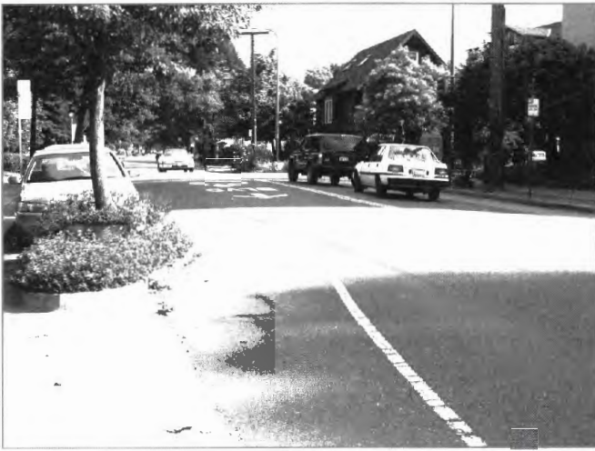
Mid-block alignment shifting parallel parking from one side to the other.
