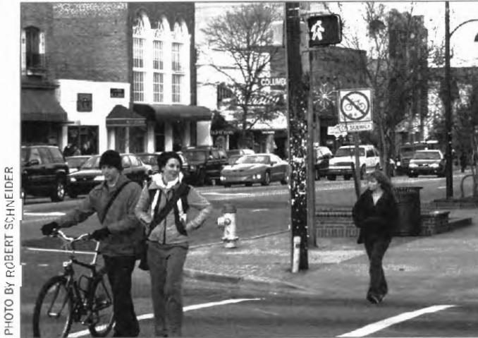
Pedestrian signals should always be clearly visible to the pedestrian while in the crosswalk and waiting on the far side of the street.
