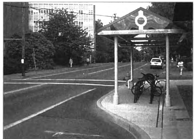
Sidewalk bulb-out with covered bike parking.
