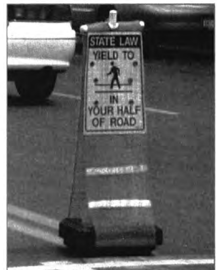
A SPCCD was placed at a ladder crosswalk on Fall Street in Downtown Seneca Falls, New York.
