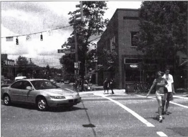
Pedestrians are quite often in conflict with left-turning vehicles when permissive signal phasing is used.
