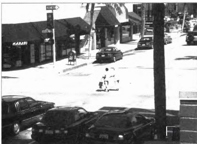
With exclusive pedestrian signal phases, diagonal crossings are allowed as well as conventional crossings.
