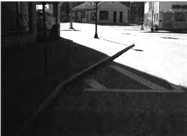
Curb extensions provide significant increased sidewalk space on Main Street.
