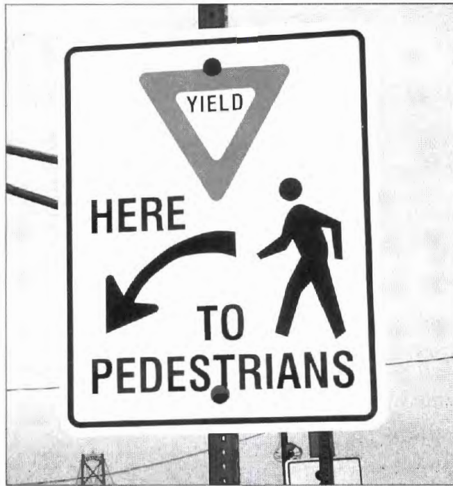
A YIELD HERE TO PEDESTRIANS sign.
