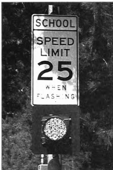
Flashing school zone beacons complement the in-roadway crosswalk warning lights.
