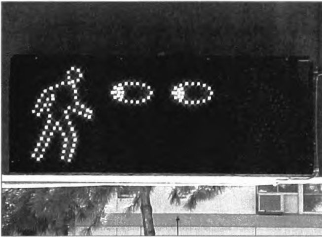
Illuminated eyes look back and forth at a rate of 1 cycle per second; the illuminated pedestrian icon (right, left or both) indicates from which direction(s) pedestrians are approaching.
