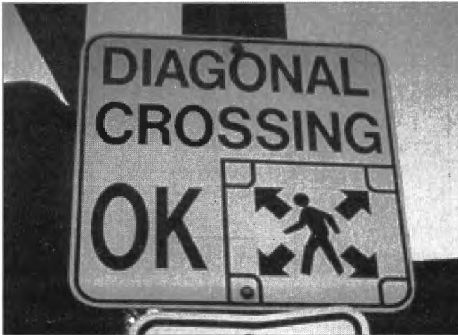
The pedestrian has a dedicated walk phase at this intersection of a busy street and a trail crossing.
