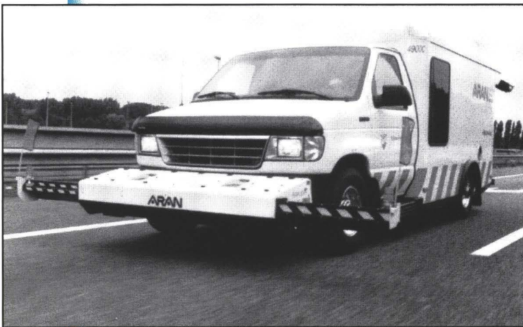
Figure 22. Surveying with the ARAN test vehicle in the Netherlands. (Photo Source: DWW, The Netherlands)
