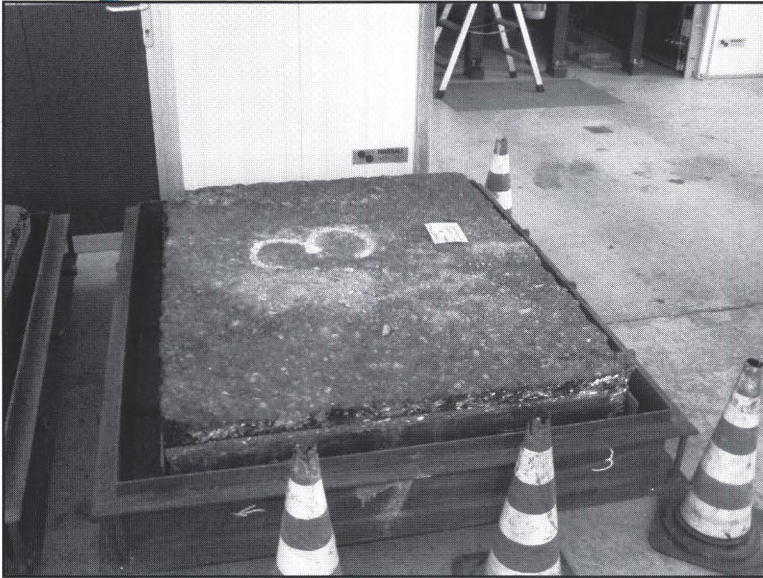
Figure 7. Block samples for accelerated loading facility testing in Denmark.
