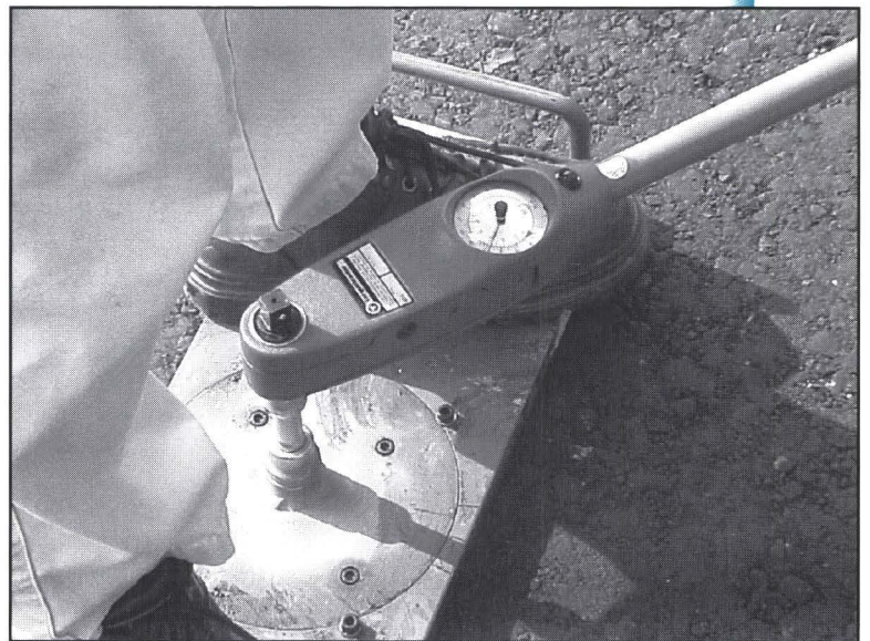
Figure 20. Use of the torque bond test in the United Kingdom. (Photo Source: TRL Limited, UK)
