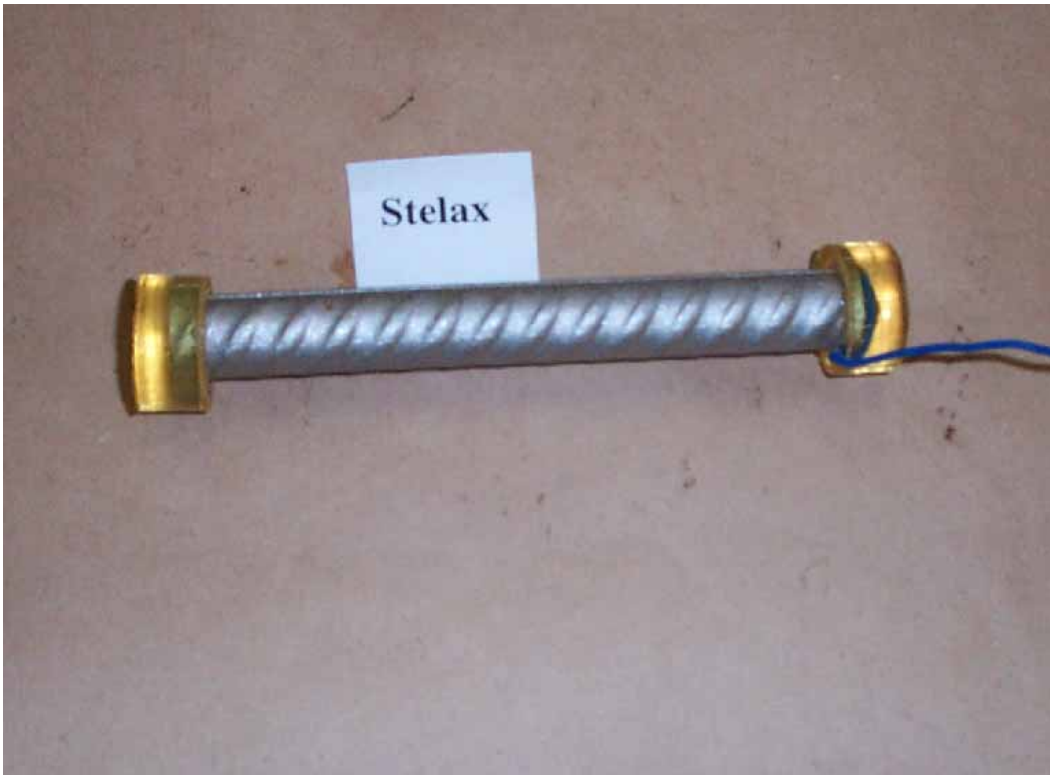
Figure 3.1. Photo. Straight, as-received, Stelax bar with epoxy-mounted ends and electrical lead.
