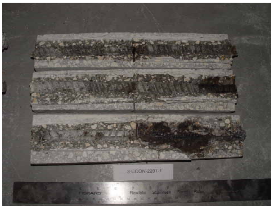
Figure 4.109. Photo. Trace of the upper rebars and corrosion products on specimen number 1-CCON-2201-1.
