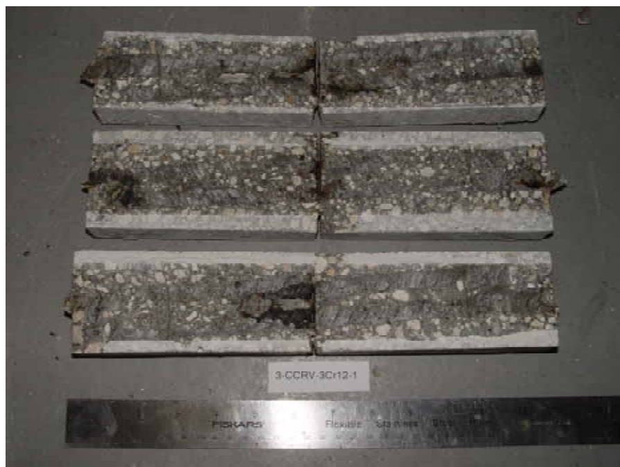
Figure 4.87. Photo. Trace of the upper rebars and corrosion products on specimen number 1-CCRV-3Cr12-1.
