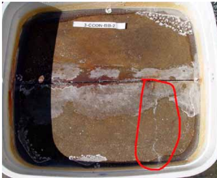
Figure 4.37. Photo. Exposed surface of specimen number 3-CCON-BB-2 after 377 days.
