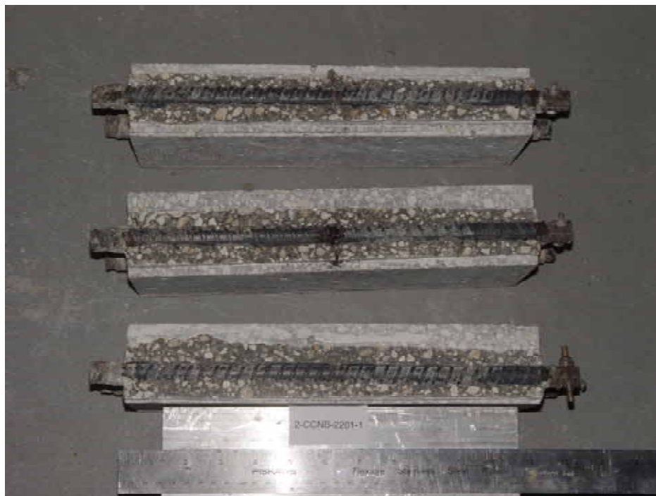
Figure 4.111. Photo. Trace of the upper rebars and corrosion products on specimen number 1-CCNB-2201-1.
