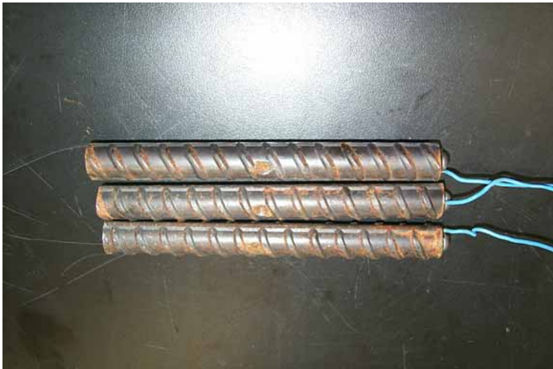
Figure 4.15. Photo. MMFX-II™ damaged specimens subsequent to AST-1 testing.
