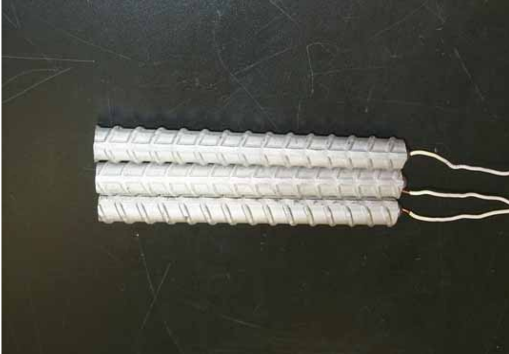
Figure 4.10. Photo. Type 316 SS specimens subsequent to AST-1 testing.
