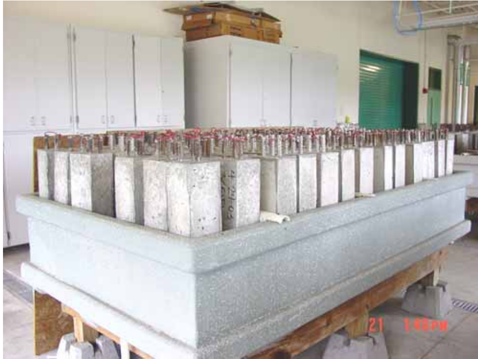
Figure 3.23. Photo. Three bar column specimens under exposure.
