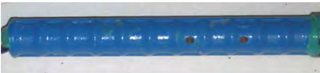
Figure 12. Photo. Bare MC anode bar with only epoxy penetrated, at 15 weeks, showing corrosion products that formed at holes through the epoxy.
