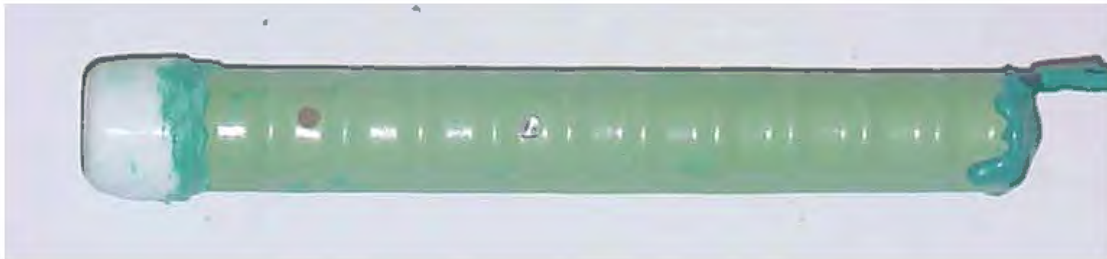
Figure 11. Photo. Bare ECR anode bar, at 15 weeks, showing corrosion products that formed at holes through the epoxy.
