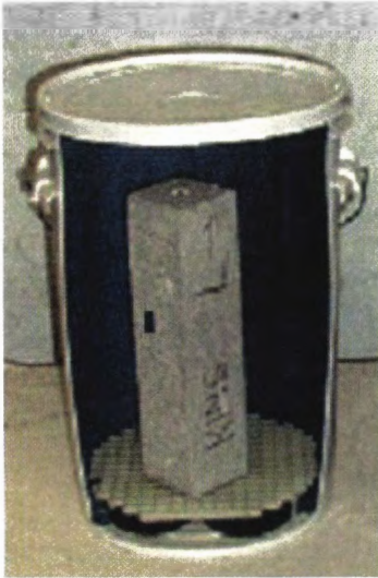
Figure 10. Concrete prism test—prisms stored over water in sealed containers.
