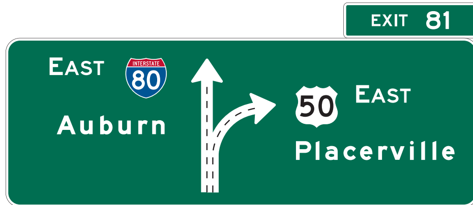
Figure 2E-7. Diagrammatic Guide Sign for a Multi-Lane Exit with an Option Lane
