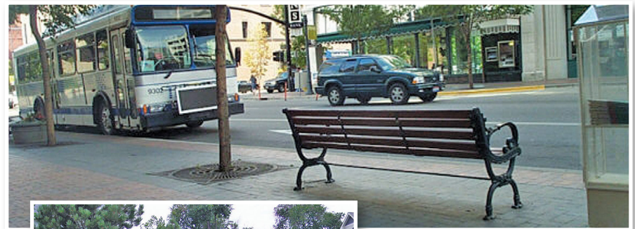
Above: Example of a bench-only stop in Boise, Idaho. The bench is not located on the bus stop boarding and alighting area and does not impede access to the stop. Source: G. Araki.
