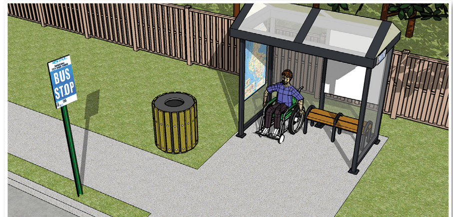
This bus shelter is placed on a concrete slab that is level with the sidewalk. It provides eight feet perpendicular to the curb, including the space within the shelter for easy maneuvering with a wheelchair. Source: Tindale-Oliver & Associates, Inc.
