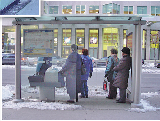
These two shelters in Toronto, Canada, open onto the sidewalk to provide protection from snow or water splashed by moving cars. The shelter is enclosed except for the entranceway to protect against inclement weather. Source: SUNY Buffalo
