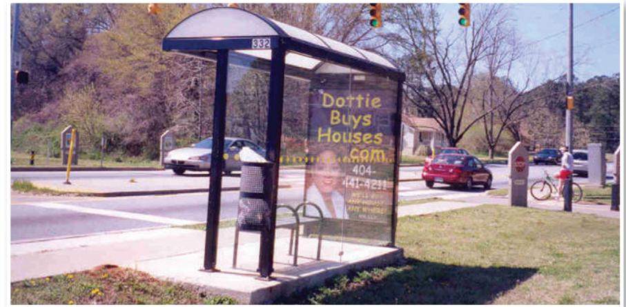
This bus shelter in Mableton, Georgia is placed on a concrete slab that is level with the sidewalk and provides a firm, stable surface for people using wheelchairs and does not obstruct the bus boarding and alighting area. Source: G. Araki
