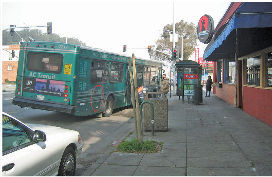
The parked car leaves little clearance for the bus to pull in flush to the curb in Oakland, California. Source: Nelson\Nygaard Consulting Associates
