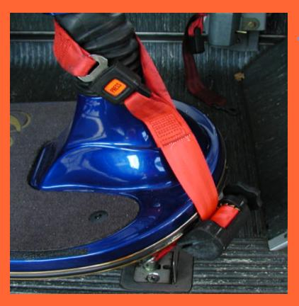
Many scooters have small wheels that do not fit into wheel clamp devices. Securing a scooter may require the use of straps placed around the wheels or frame.
