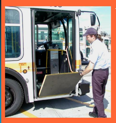
The ramp on a lowfloor bus can be manually operated in the event of a mechanical failure. The Operator simply lifts up on the strap to deploy or stow the ramp.
