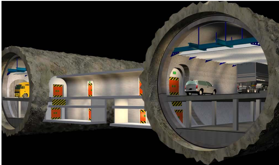
Figure 2-3 Rendering of M 30 Tunnel cross section with cross passages between tunnels for emergency use.
