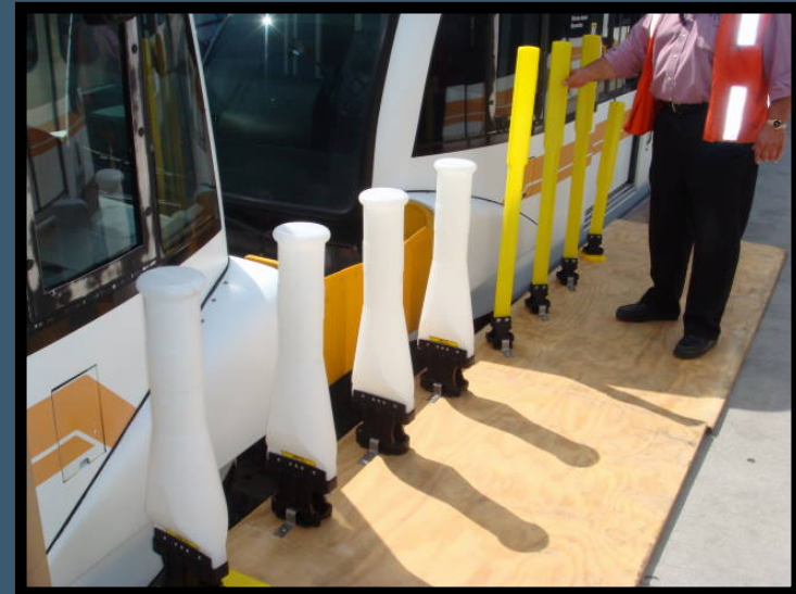
CPUC Platform Barrier Six Month Test on Gold Line
